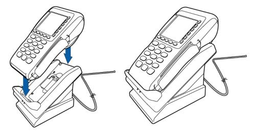
Figure 23 Placing the V<sup>x</sup>670 onto the Base Station
